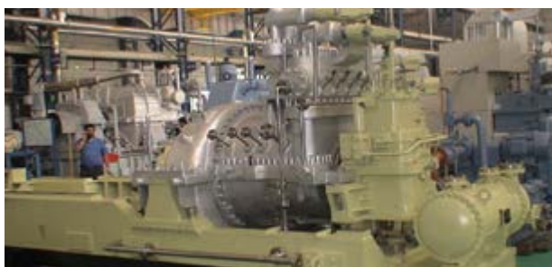
TAT (Turbo Alternator) turbine developed & supplied to DMDE by Triveni Turbines as an OEM
