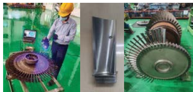
INS Vikramaditya Turbo Blower Unit gas turbine blades indigenized & supplied through reverse engineering.
