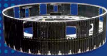
4m Dia Stiffened Structure for GSLV Mk-III
