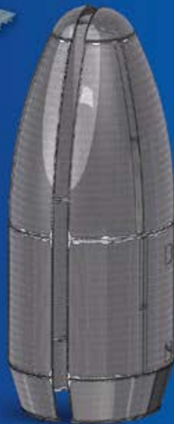
5m Dia 10.7m Height Payload Fairing Jig & Assembly For GSLV Mk-III
